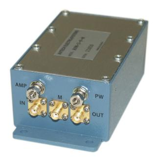
The "AMP" and "PW" controls may be adjusted using a screwdriver. Units with the -EA or -EW options will have solder terminals instead of screwdriver-adjustable controls.
